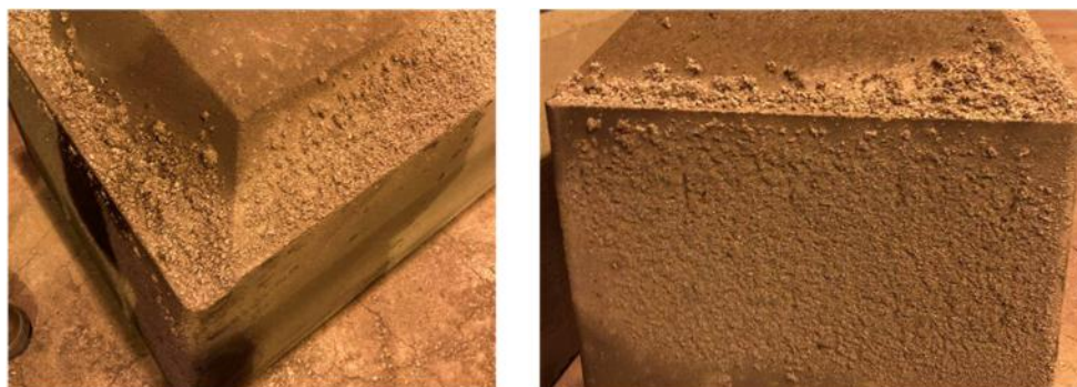
Figure 1. Sticking of packing coke to anode blocks (Courtesy of Alcoa Corporation).
